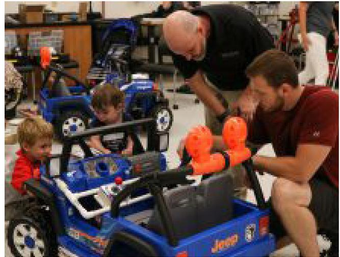
and reverse movement. To help turning, the engineering team added a single caster wheel in the front that allows effortless turning in any direction. To increase safety, a harness system made from PVC pipe and foam padding was implemented.
